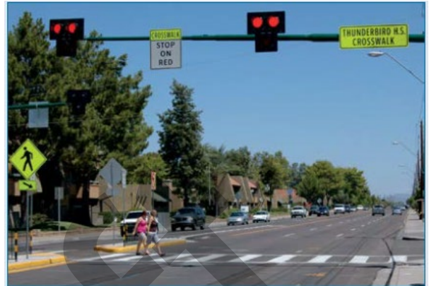
HAWK signal in Phoenix, AZ. Source: U.S. DOT FHWA.
